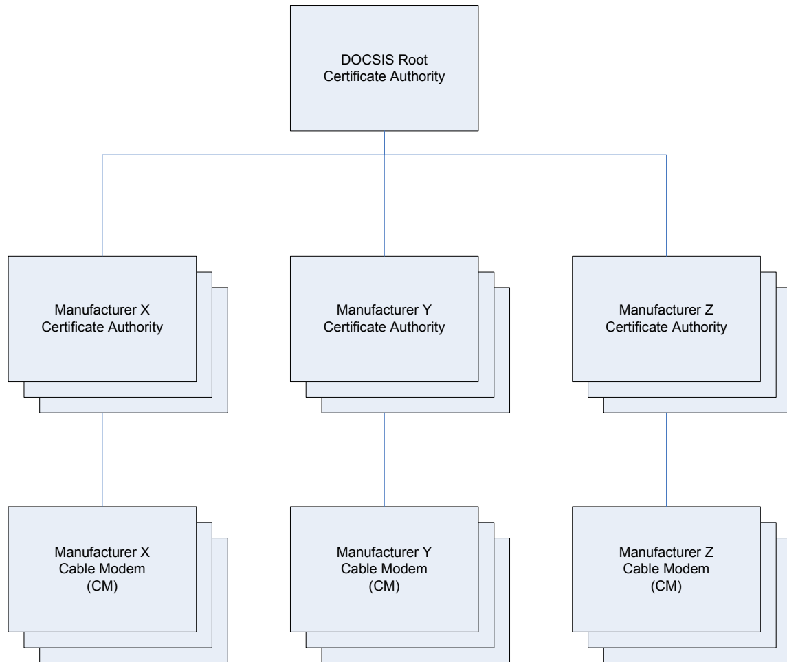
Figure 13-2 - The Distributed Model of the DOCSIS Certificate Management Architecture
